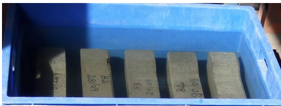
Typical water absorption test
